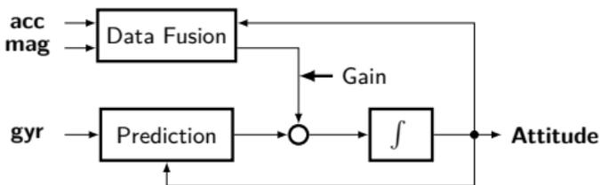
Attitude estimation principal schema using an accelerometer, a magnetometer and a gyroscope.
