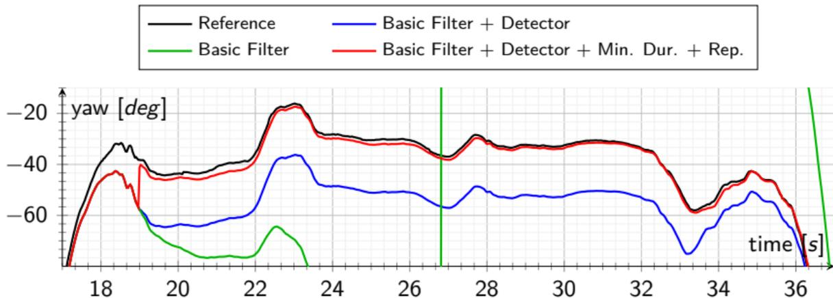
Sample run of the reprocessing technique (red) when a magnetic perturbation occurs, in comparison to ground truth (black) and earlier techniques.
